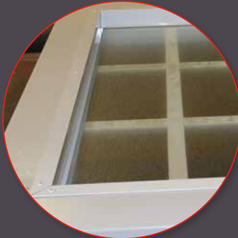
Glass is sealed with bonding tape around perimeter of window and on back of grid, providing superior weather protection and making field painting much easier. Glass is secured with prepainted aluminum trim on interior of door
