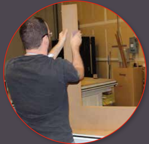
Overlay receives final inspection and prefinish sanding before applying
